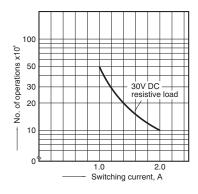
3. Mechanical life Tested sample: TX2-5V, 10 pcs. Operating speed: 180 cpm
