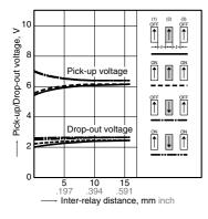
4-(2) Influence of adjacent mounting Tested sample: DS2Y-S-DC12V, 10 pcs. Ambient temperature: 20°C 68°F
