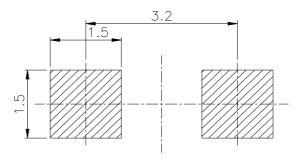
**Note:** The tolerance unless mentioned is  $\pm 0.1$ mm, unit is mm
