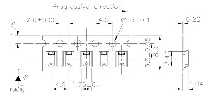
**Note:** The tolerance unless mentioned is  $\pm 0.1$ mm, Unit is mm
