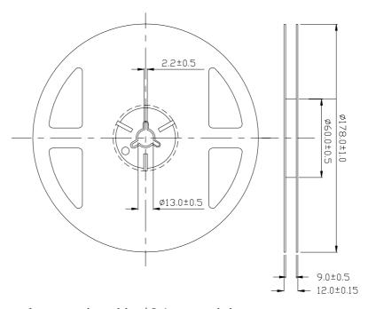
**Note:** The tolerance unless mentioned is  $\pm 0.1$ mm, unit is mm
